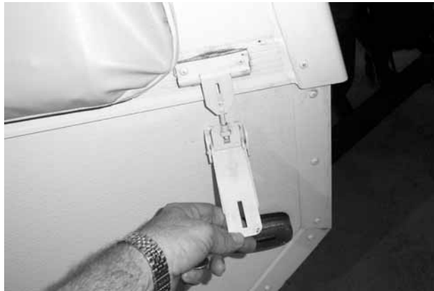
Prior to raising roof, unlatch all four corner latches.
