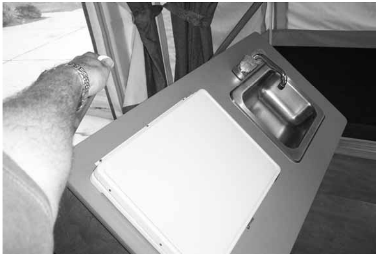
Raise Galley into position.
