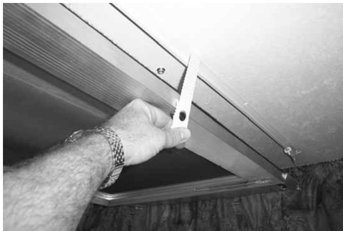
To lower screen door, first release two snap straps.
