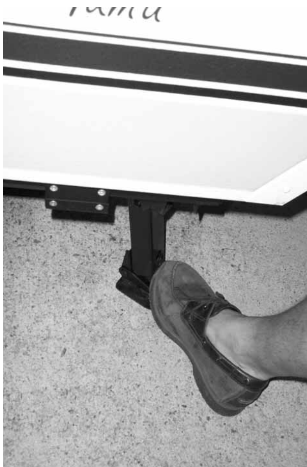
Before lowering roof, release all jacks.
