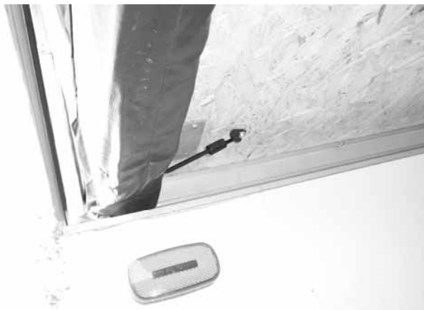
Another REMINDER - REMEMBER TO UNHOOK all bungee cords BEFORE BEDS ARE PUT BACK! EXPENSIVE DAMAGE WILL OCCUR TO TENTING FABRIC!
