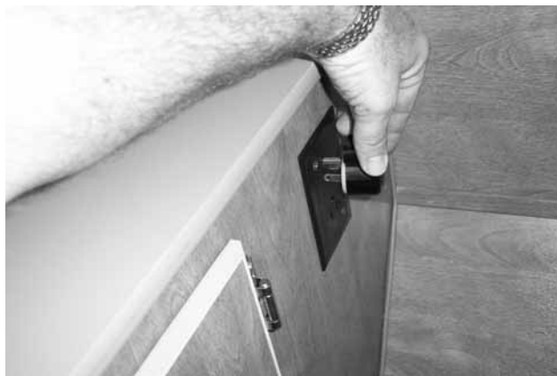
At set-up Plug in A/C power cord in outlet. Air Conditioner cord stows at ceiling under curtain with VELCRO. MAKE SURE TO STOW ON TAKE-DOWN BEFORE PUSHING IN BEDS.
