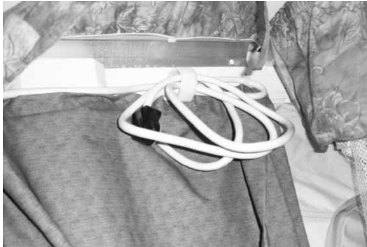
Air Conditioner cord stows at ceiling under curtain with VELCRO. MAKE SURE TO STOW BEFORE PUSHING BEDS IN!
