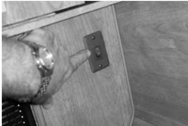
Turn on Water Pump switch. Turn OFF when traveling.
