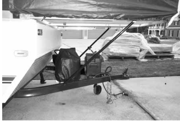
Pull out front bed and lower bed support rails. Attach to frame rail studs.
